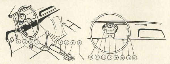
1, Lights and dipswitch. 2, Direction indicator control. 3, Cold air intake control. 4, Horn button. 5, Gear lever. 6, Handbrake. 7, Choke control. 8, Starter switch. 9, Heater
