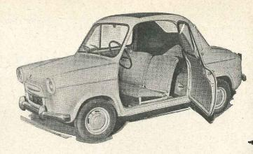
Two adjustable seats and extra space usable for luggage or children (with an optionally available cushion) leave plenty of room for the longest-legged driver. The on-off control for the heater is visible behind the seat.
