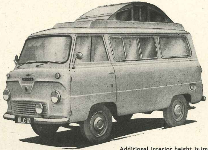
Additional interior height is imparted to the Ford Thames conversion by an elevating roof, shown here in the raised position. The curtains offer privacy.
